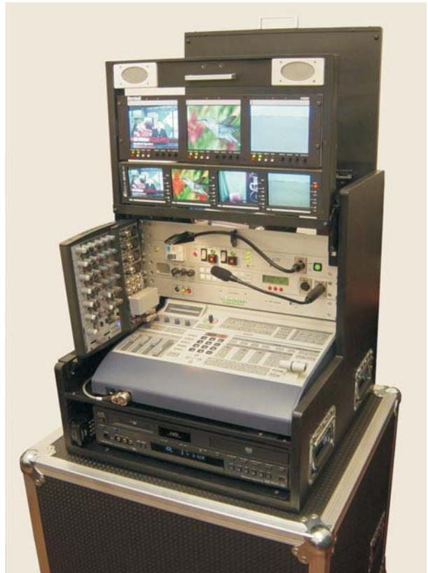
The inputs of the same cameras can be used in its turn as digital VCRs. Moreover, thanks to installed "3 in 1" JVC SR DVM700 professional VCR it is possible to use material shoted on the following supports: DVD, mini DVD and mini-DV.
